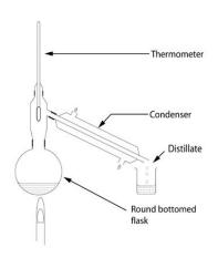
In the AromaLab, distillation methods rely on the water cycle. Because we can control when the water is in gas form or liquid form, we can also control its ability to carry a scent from a raw material into the product.
